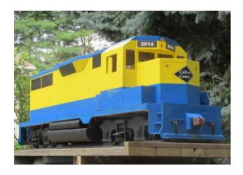
This is the 'Calvert-Central' GP35. Made mainly of plywood, it boasts 2x 350-watt motors geared through chains in the bogies. Rather intriguing ideas used in this! See more at http://calvertcentral.com.
