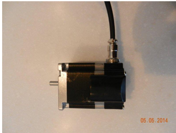
Photo 8 Motor with end cover & plug fitted up this is a slightly smaller stepper motor. The 175 oz one I had to modify the cover a bit to get it to fit around the plug.
