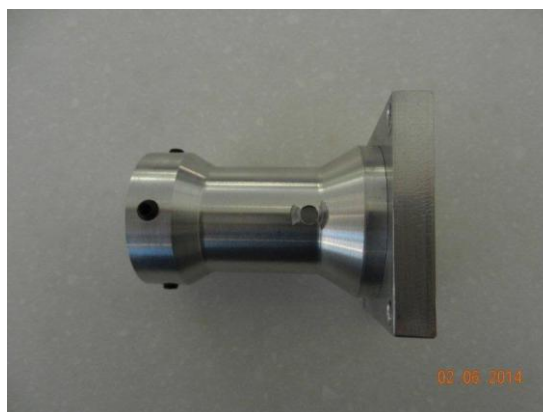
Photo 7 The custom motor to table connection, found this shape on a You tube video & thought it look rather nice.
